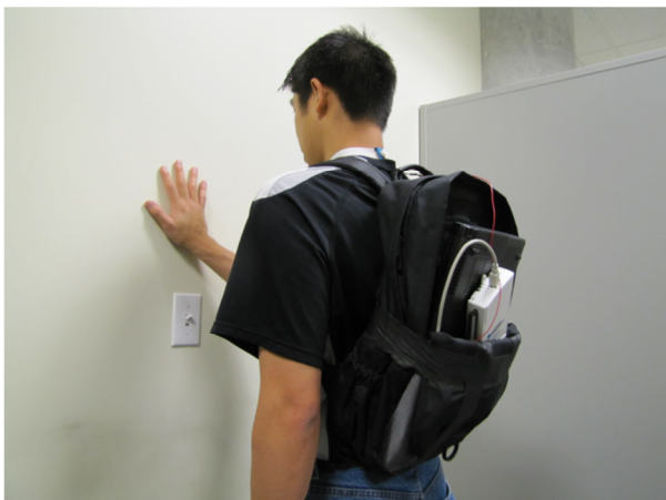
Figure 2: Experimental setup. A laptop and a USB data acquisition device are worn in a backpack. A wire connects the data acquisition device to a conductive pad in contact with the back of the participant's neck.
